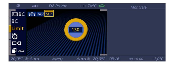
The range above this speed is displayed with a bright bar segment within the speedometer dial in the LCD area of the speedometer.
